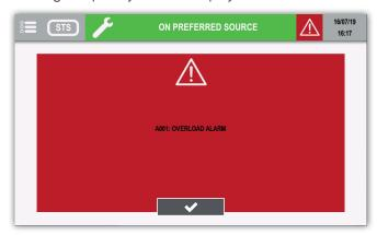
Tap on valid button to stop the buzzer and to close the popup message. The alarm page is automatically display after this action.
